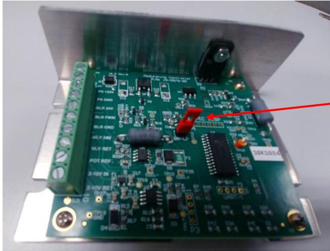
Insert the Jumper in the two pins on the Controller
