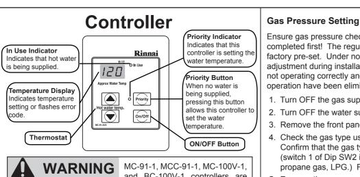
and BC-100V-1 controllers are not compatible with Alternate Temperature Settings. Alternate Temperature Settings are for commercial applications only. DO NOT use the MC-91-1, MCC-91-1, MC-100V-1, or
