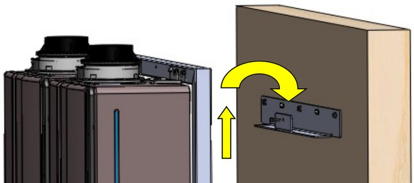
**3** Secure the front of the bracket to the front of the wall hanging frame with a #12 X 3/4 drill point screw.
