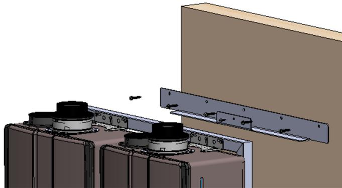
**2** Lift the wall hanging rack and insert the top of the frame into the bracket.
