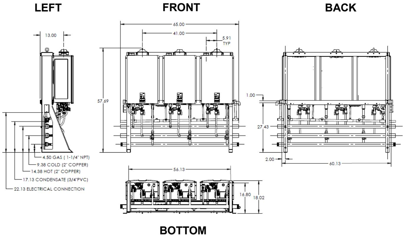
The above configuration is a 3-unit wall-mount frame which is available as a custom, made-to-order (MTO) solution with extended lead times.
