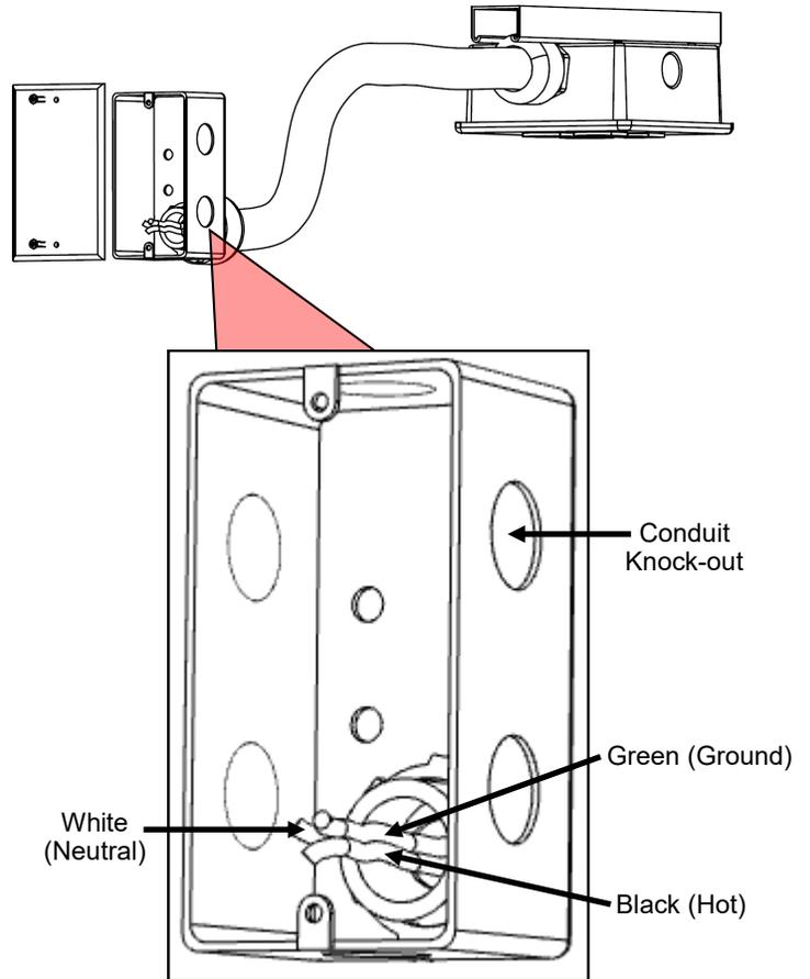
1. Locate the gang box on the side of the TRS frame.
