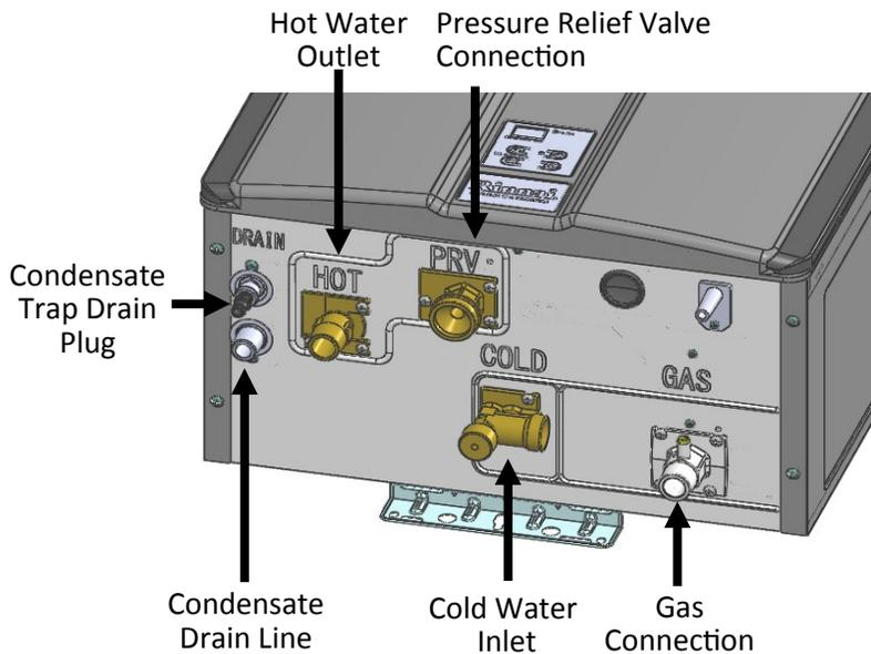
The condensate drain pipe (along its entire length) must be at least the same diameter as the drain line.
