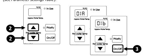
3. Once the desired setting number is selected, use the "On/Off" button on the controller to change the selection for the setting number. Example: Display will change from 01A to 01b for Maximum Temperature setting (as shown below).
