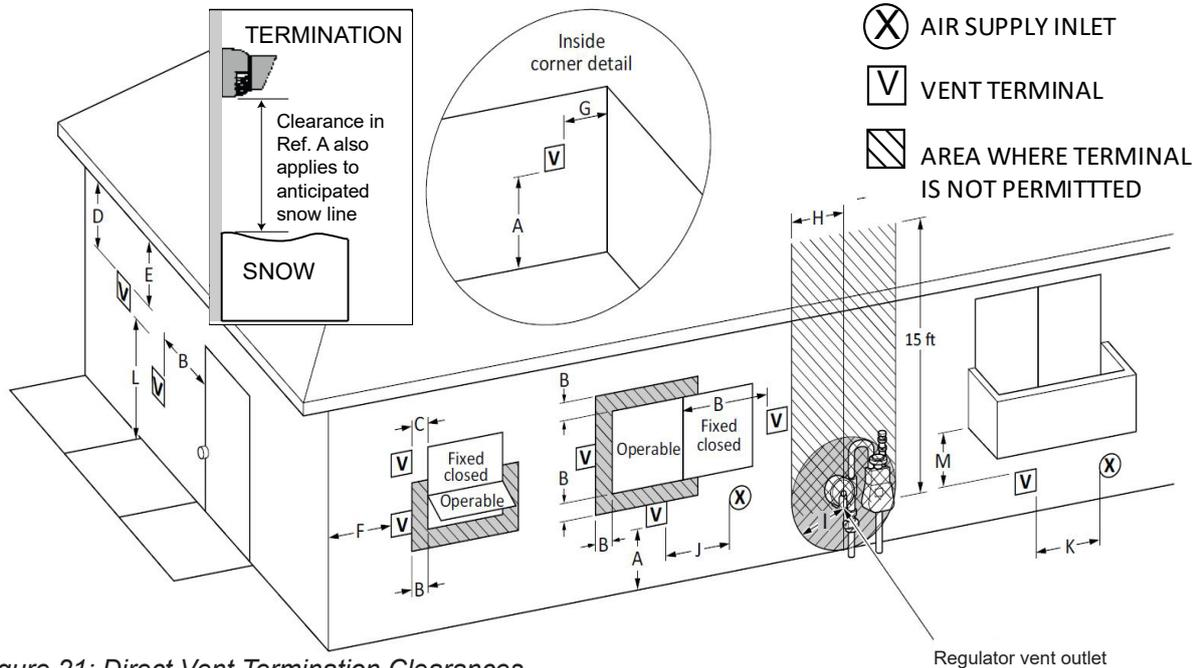
Figure 21: Direct Vent Termination Clearances
