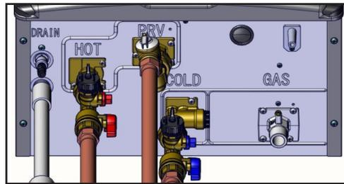
Figure 48: Pipe connections on bottom of water heater
