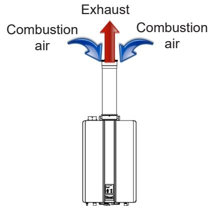
Figure 23: Concentric Pipe
