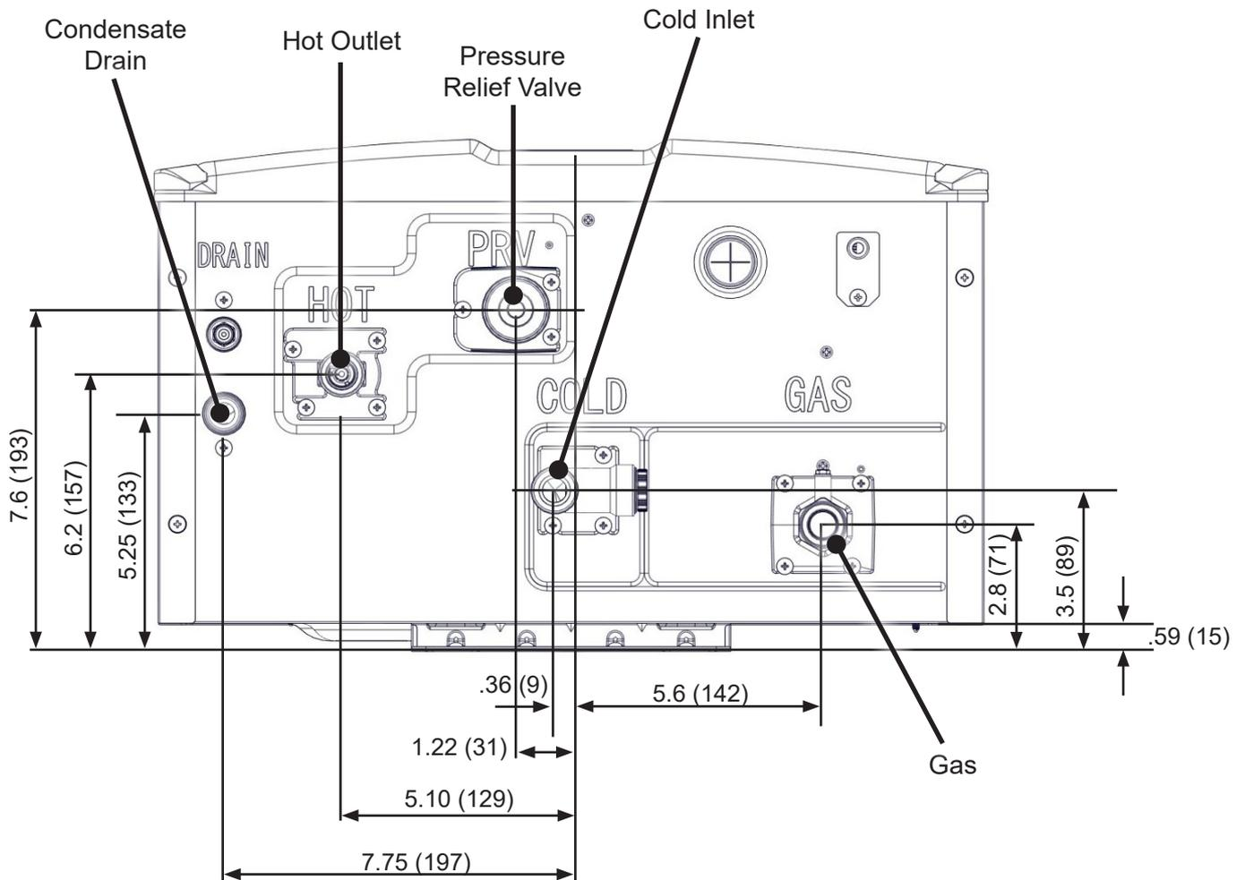
Figure 6: Supply Connections
