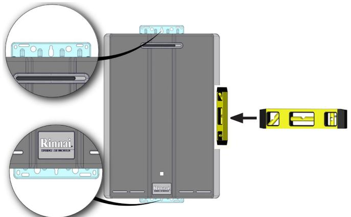
Figure 13: Mount water heater
