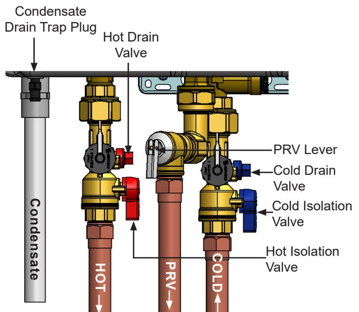
Figure 79: Piping Diagram
