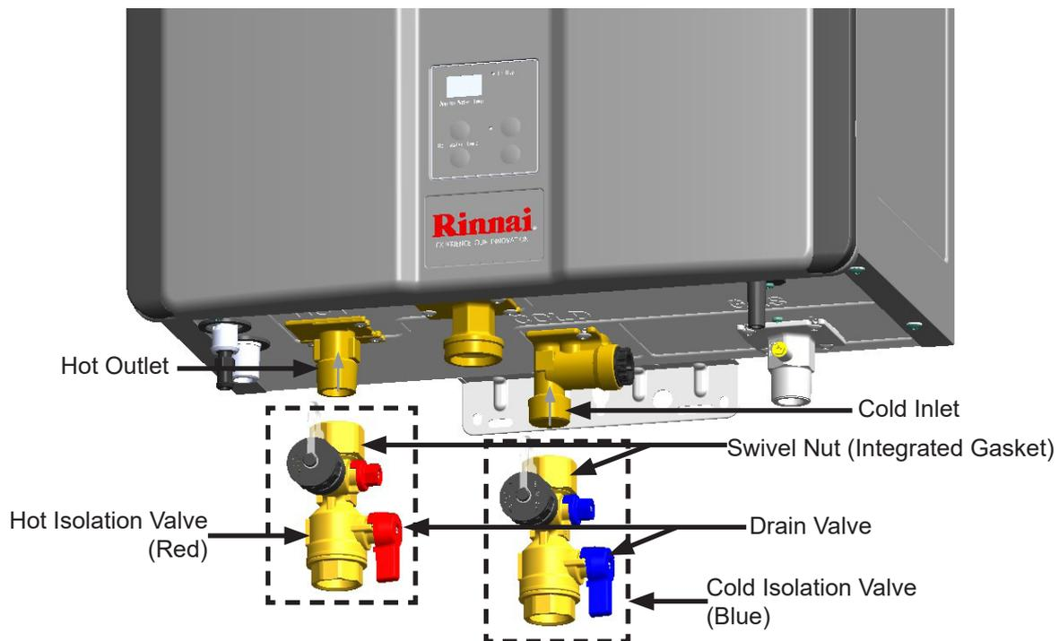
Figure 52: Install Isolation Valves
