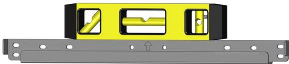
Figure 9: Level the bracket
