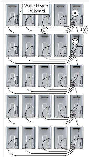
In the diagram above, 25 water heaters are electronically connected. Each bank of 5 is controlled by an MSB-M control board. These boards are connected to each other with MSB-C2 cables. One MSB-M is the controlling or master MSB-M for the entire system.
