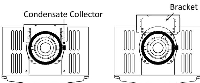
To adjust the condensate collector position or to replace the female vent top with a male vent top:
