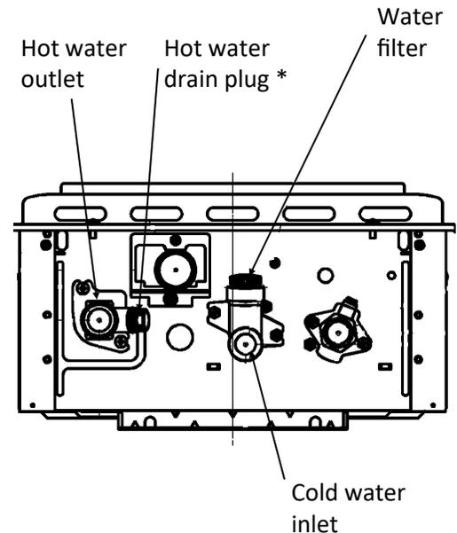
\* Use a wrench or other tool to unscrew the hot water drain plug.
