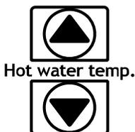
3. Press the up or down buttons to obtain the desired temperature setting.
