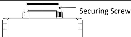
Secure the first vent component to the water heater with one self-tapping screw at the hole located above the condensate collector.
