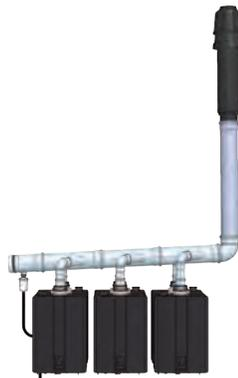
**ROOM AIR COMMON VENT CONFIGURATION VERTICAL EXHAUST CU199 ONLY**
