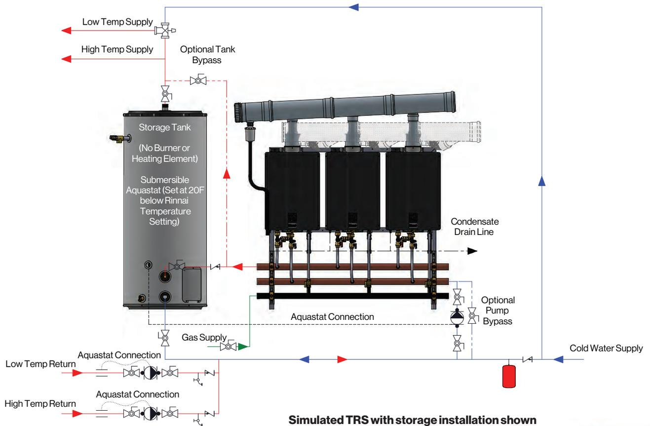
Flexible installation is another TRS strong suit. It fits through a standard 32" doorway, has various venting options including PVC and the Rinnai Common Vent system, and can be mounted indoors or outdoors, either floor-standing or wall-mount.
