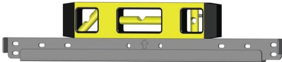
Figure 9: Level the bracket
