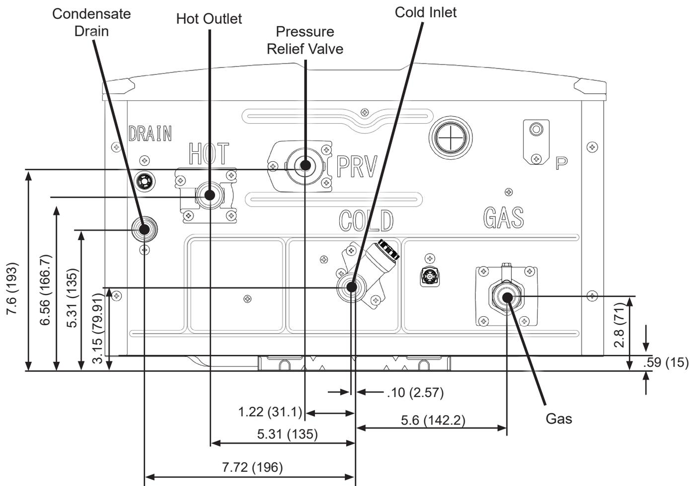
Figure 6: Supply Connections
