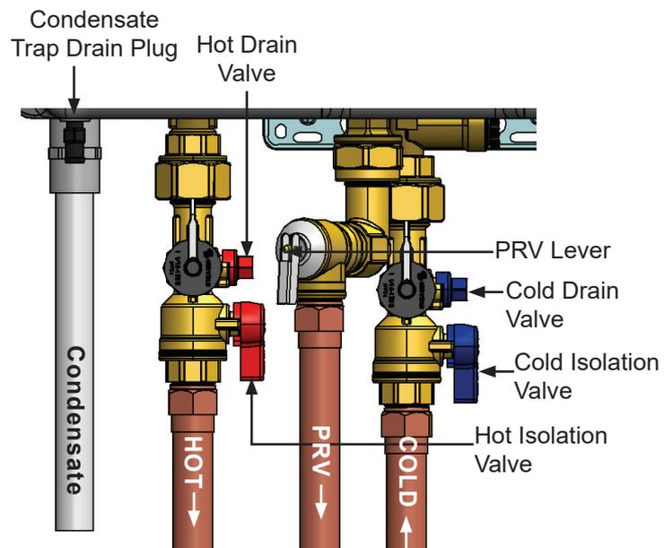
Figure 96: Piping Diagram
