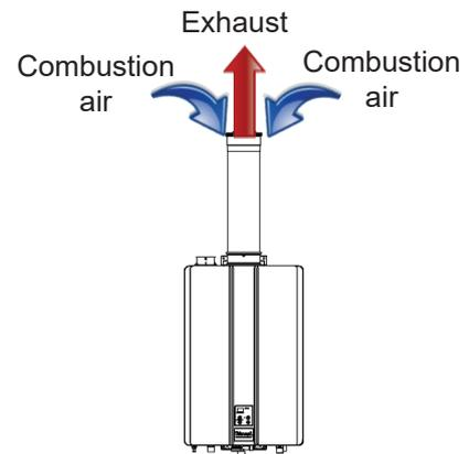
Figure 23: Concentric Pipe
